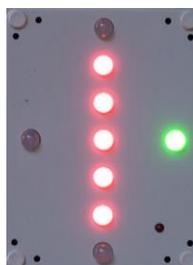
9. Just after all vertical RED LEDs turn ON, the Green Directional LEDs, and RED LEDs will be turned OFF and another audible beep will occur as the fielder releases the throw.
