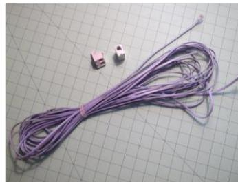
The small couplers allow the interconnection of the cable between the Timing Light and Video Option.
