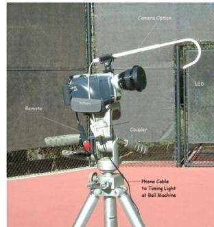
The Extension Cable Option can be purchased (see pricing sheet) and will allow the video camera to be located up to 100 feet from where the **Ball Machine Timing Light** is located.
