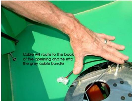
13. Route the phone cable down the rear-left side (as reference when standing & facing the front of ball machine) being sure to keep the cable as close to the metal side and away from the rotating wheels and motors. Cable damage can occur if not properly routed.
