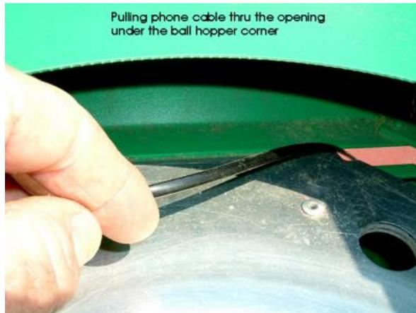
11. Continue routing around the feed 'wire' ball hold down post and towards the left side of the ball machine (the side with the control panel). Locate the 3 Stick Downs on the cable and clean the aluminum plate with a rag so that you can secure the cable by removing the paper tabs from the 3 Stick Downs. A tie wrap can be used to secure the cable to existing electrical cable at the back of the carousel being sure to keep the cable away from the carousel's path.
