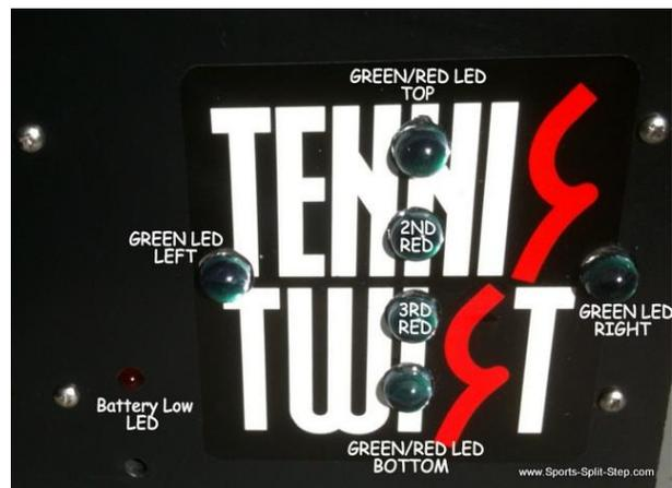
Close Up of Timing LEDs
