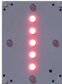
3. After all the LEDs go OFF a beep will occur and the pitcher releases the ball; as the vertical RED LEDs begin moving upward, the batter begins their stride forward.
