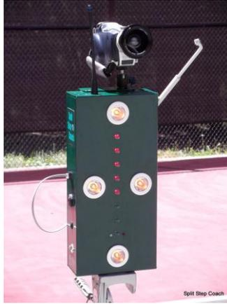
2. [A Timing Device & video camera](#) used with the Split Step Coach allows measurements of athlete's performance. The Split Step Coach can be operated at the baseline, net or from your ball cart.
